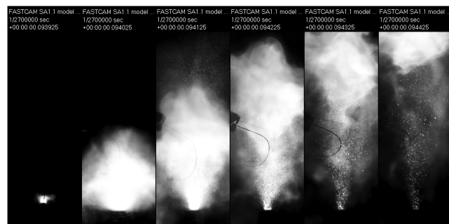
Fig. 10 Sequence of high-speed video frames from a thruster tested in the fast regime with the motor without a nozzle. There is 100 \mu s between each image (total time is 500 \mu s).
